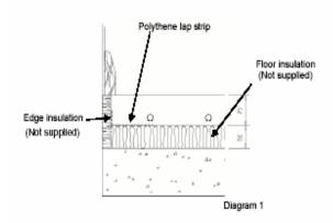
Note, some insulation board manufacturers recommend that you tape the joints to prevent screed ingress, which can form cold bridges.
