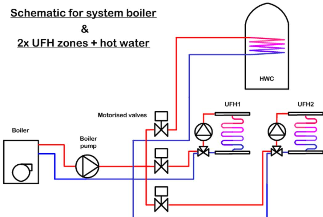
**Schematic for system boiler
