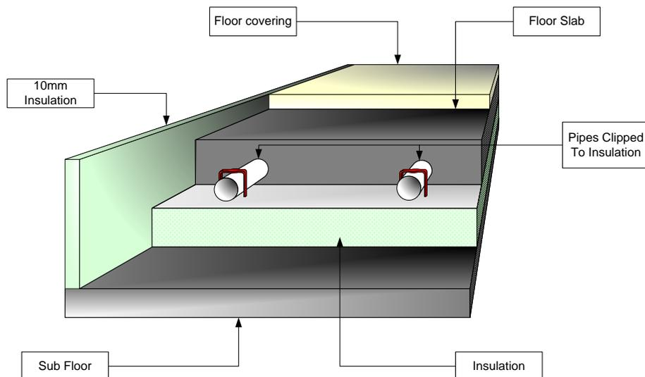
The Underfloor Heating system can be fitted in both concrete and timber suspended floors. See picture above. For other floor constructions please contact us and we will explain installation procedure, for
