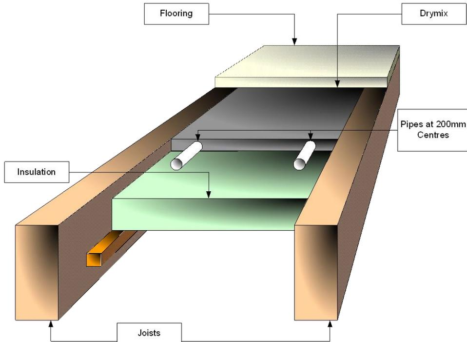
The Drymix is needed for Ground Floor, older buildings and if concrete floor and timber suspended floor are on the same floor. **For First Floor applications when property is built to current building regulations an air gap is fine, still good to use the drymix as will give out more heat.**
