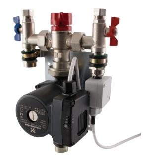
Designed for use on small rooms or extensions, provides temperature controlled mixed water to underfloor heating systems with a heat output of up to 3kW, satisfying underfloor heating areas upto 40 sqm.
