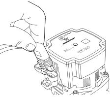
To comply with IEE regulations, the pump on the Thermoguard UFH Control Pack must be provided with an earth. All wiring should be undertaken by a qualified installer and must conform to IEE regulations.
