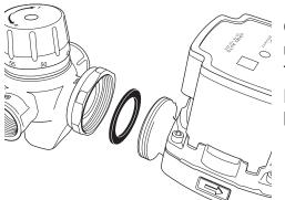
Connect the Thermoguard UFH valve to the pump using the pump nut which is pre-assembled to the Thermoguard, ensuring the pump washer is inserted. Please take note of the directional arrow on the pump body.
