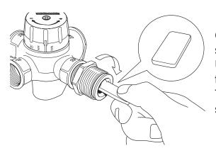
Once the orientation has been determined the straight connector which connects the Thermoguard UFH valve to the manifold needs to be screwed into the return port.
