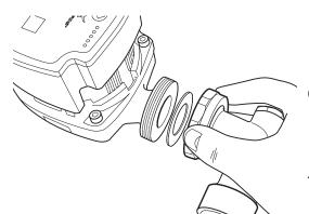
Connect the nickel plated elbow to the pump using the  $1 \frac{1}{2}$ " pump nut, ensuring the pump washer is inserted.
