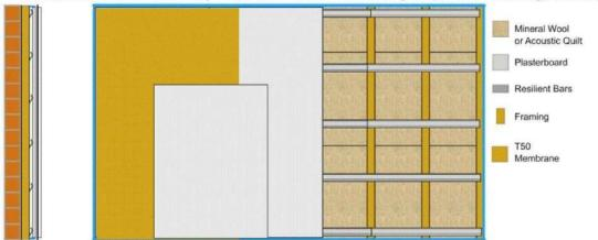
Stick up the T60 membrane then add the final layer of plasterboard offset against the first
