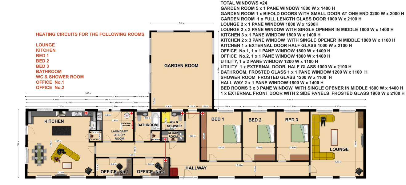
EXTERNAL WALL 140mm INTERNAL WALL 140mm
